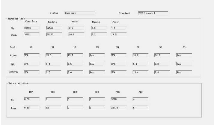
Pic 7.4-1 Physical layer data
